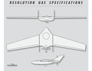
Gross Weight : 10 lbs Useful Load: 4-5 lbs Wingspan: 7 <sup>1</sup>/<sub>2</sub> ft (2.3m) Rate of Climb: 500 fpm Cruise Speed: 25-75 kts Survey Altitude: 500-1500 ft
